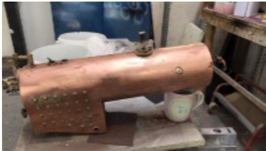
The boiler stripped and cleaned
