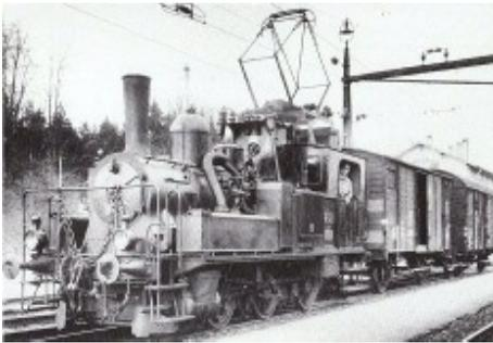
When the Swiss Railways were electrified, to avoid having to replace the Station Pilots, these were fitted with a pantograph on the cab roof and the boiler converted to electric heating. This made them pollution free, though at the time this was not a cause for concern!
