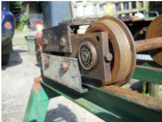
The same bogie with the anti tip angle in place
