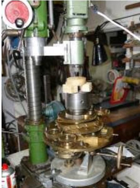
The chuck mounted on the Mill
