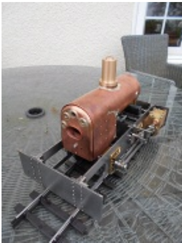
The frames with the part built boiler
