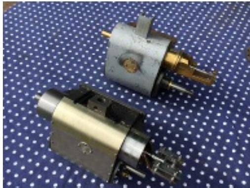
the oven saw them removed only to reveal a very poor finish to the components with insufficiently sized steam passages to make the thing work effectively. A known Winson fault. Should I machine the old castings and fix the valve liners or buy new ones that looked more like the real thing? New cylinder castings were ordered from Doug along with the detailed castings for the front and rear cylinder covers. The cylinders and driving wheels were superbly machined
