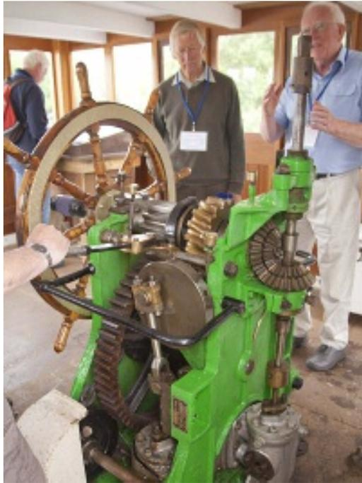
The restored steering engine and manual ship's wheel.
