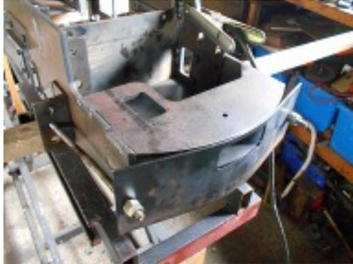
The method used to form the bow ends
