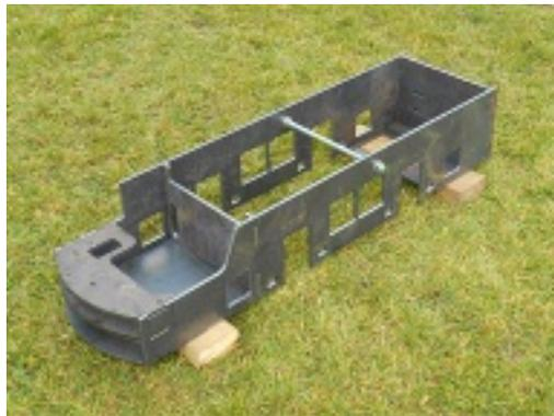
and temporarily assembled to check the CAD.
