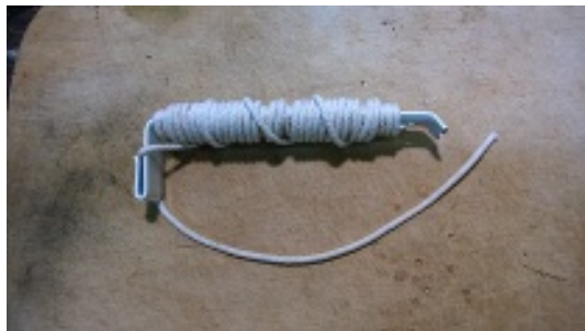
A shuttle for winding string on pipes still attached to the engine
