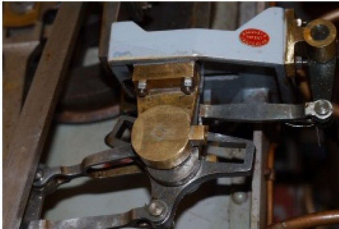
The Baguley valve gear on "Sanford" and the plate.
