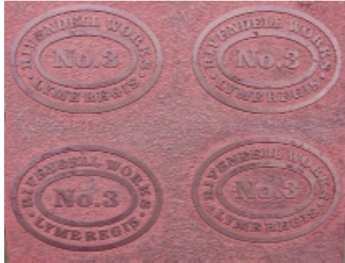
Plates with the resist removed (pic 4)
