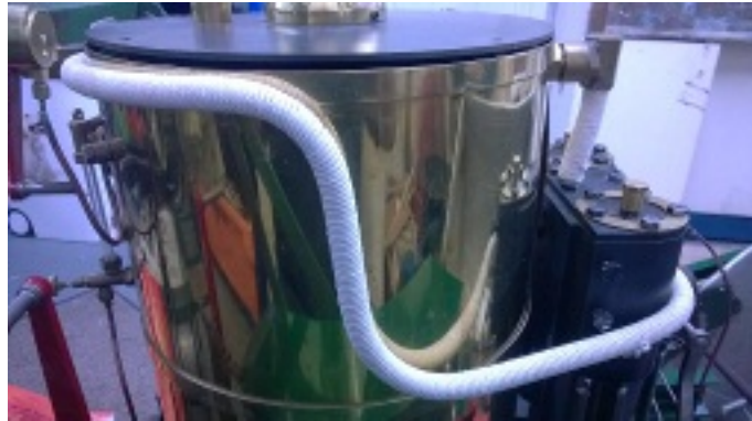
Viewed from the right, the steam delivery pipe and exhaust pipe lagged as described.
