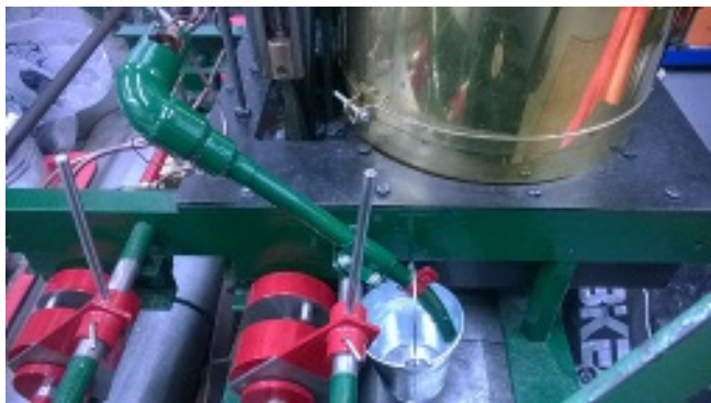
Viewed from the left the cylinder drain collector pipe and the galvanised bucket
