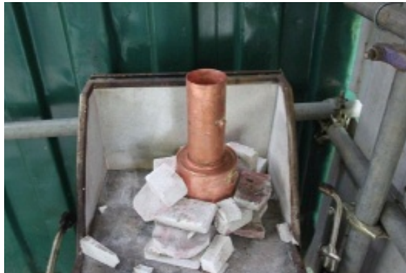
A part built boiler on the brazing hearth
