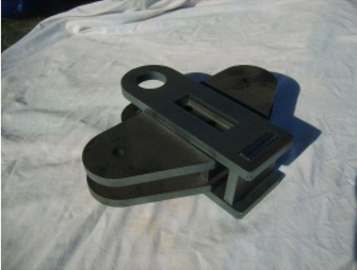
The plates were laser cut from 12mm. mild steel. The photo shows the parts as they arrived and in much the position they will be when the rest of the bits have been made and the whole thing assembled. Even without the rollers this is a heavy piece of kit. The intention is that it should be bench mounted but there is no reason why it could not be mounted on a suitable truck, if this turns out to be more convenient.
