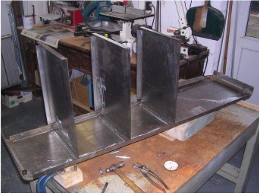
Part built showing internal baffles
