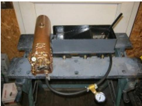
I then made a T-piece to insert the gauge midway along the high pressure hose and connected this to the tender pump and boiler, as can be seen in the photograph. I was now able to pressure test my boiler and establish where any leaks were, allowing me to correct any silver soldering problems.
