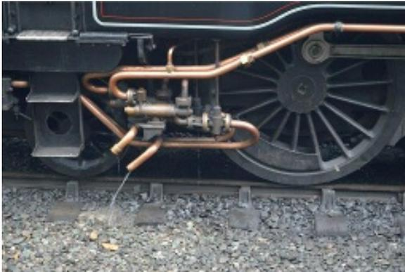
A 12inch to the foot scale injector earns its keep at Llangollen.
