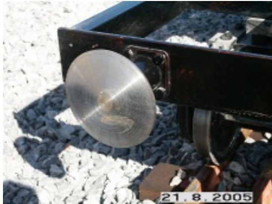
Finished buffers on the old stock
