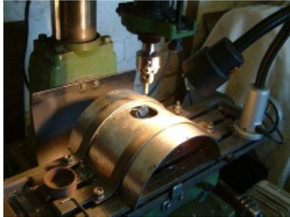
The photograph shows the setup when the boring head was being used to finish the hole to size.
