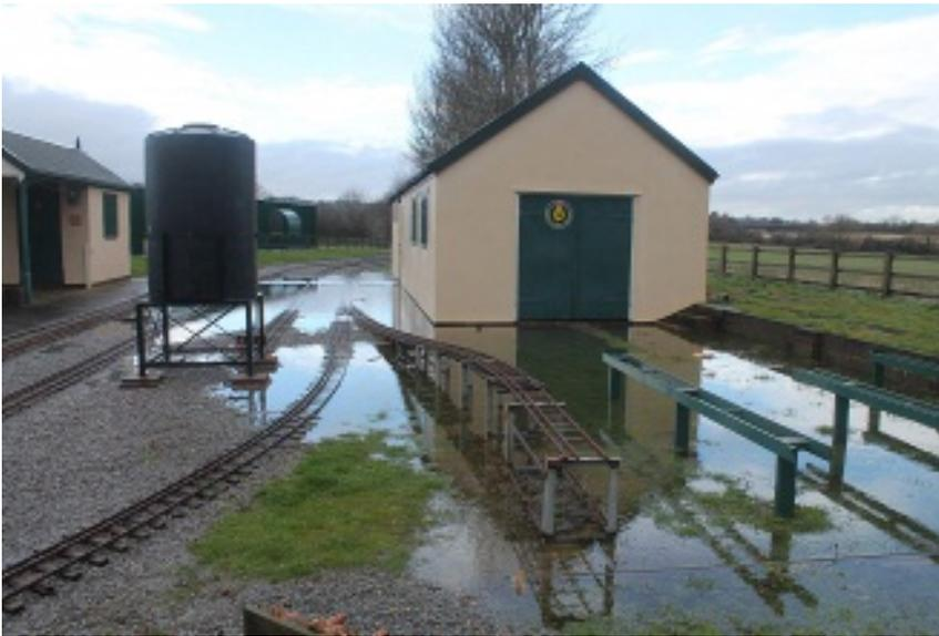
The result was that outside work stopped until the water drained away and it was possible to inspect the track and repack some of the ballast where it had been disturbed.
