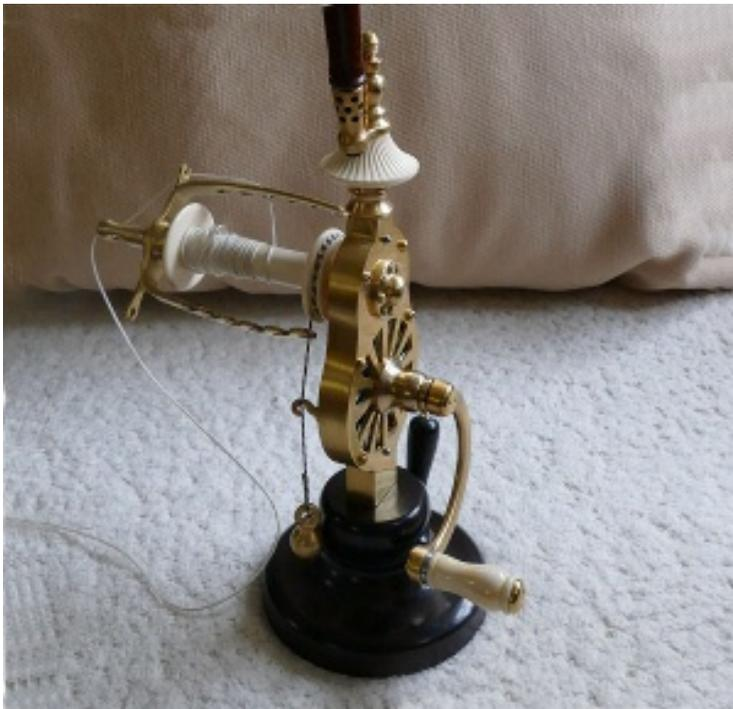
A quick search through the boxes of stuff I should have thrown away years ago turned up a pair of gears more or less the right size, these were laid out on one of the side plates and the centres found using toolmaker's buttons. The side plates are 1/8" with a 1/4" centre piece held together with 6BA screws. The rest is pretty much plain turning/filing etc. The fancy rivets are bog standard 3/32" prettied up a bit, the fancy parts are ivory and decorated on my Rose Engine.
