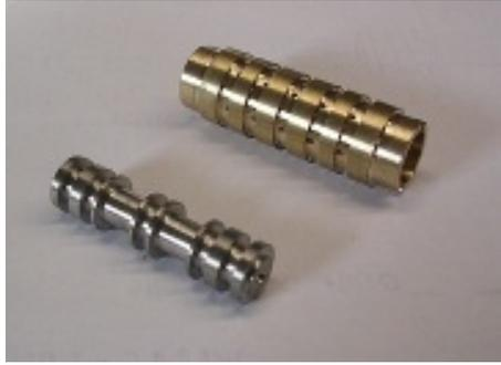
The shuttle valve components
