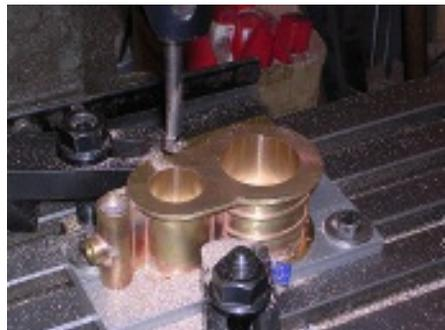
Milling the high pressure air bore
