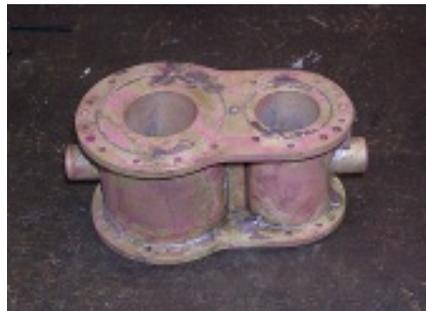
The bottom cover was next. It has various bosses and passageways on it and, as a result, bent like a banana. Which was a bit irksome. I managed to straighten it a bit and then put it in the four jaw to skim it flat and it worked out OK, fortunately.
