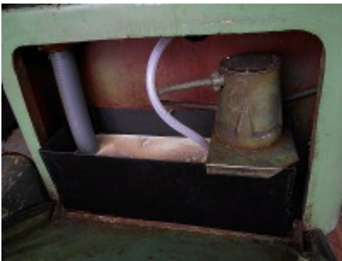
The coolant pump and tank
