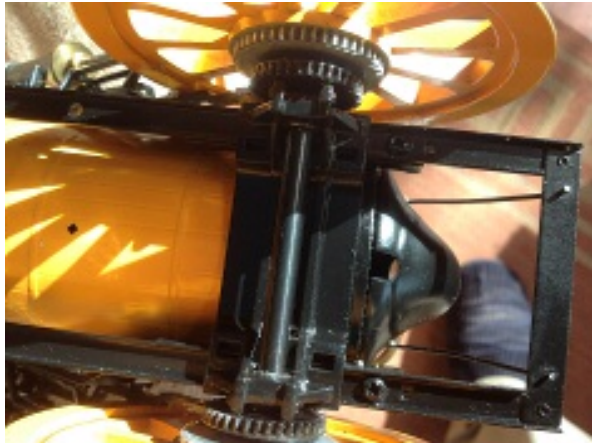
The unusual “final drive” on the “Rocket”.
