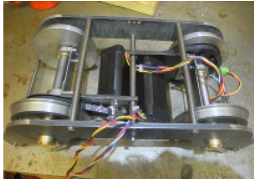
The two motors in a "Wedge" bogie.
