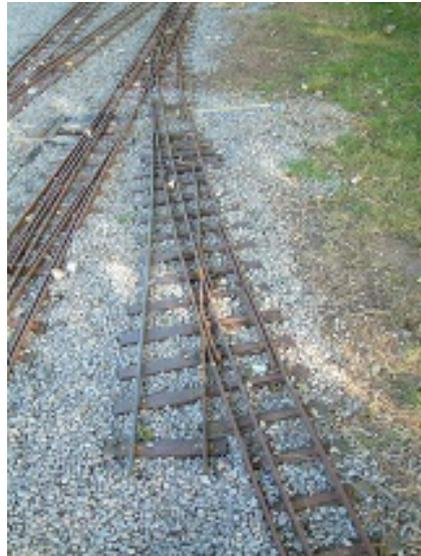
The new points with 7.25" gauge only into the carriage shed.
