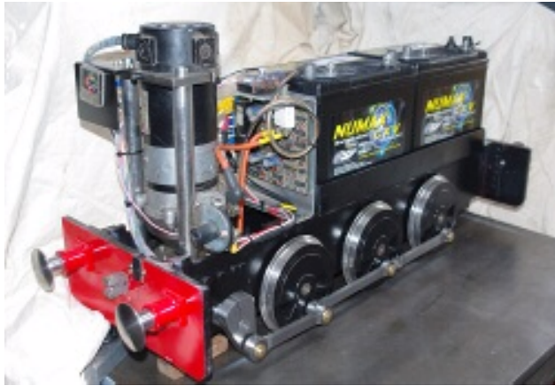
Locowithcabremoved –notthetemporary wiringarrangement
