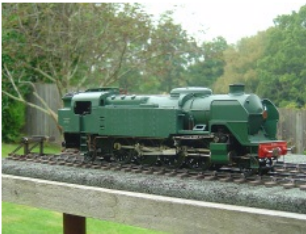
A spirit-fired suburban tank locomotive On the author's gauge 1 layout.
